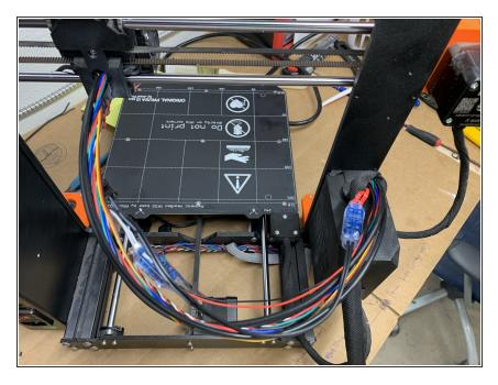
Open the wire bundle up by removing the cloth jacket all the way to the control box and exposing the full length of the heater and thermistor wires.
