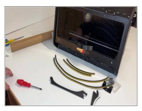
Install the side bars for the seal kit as shown here.
