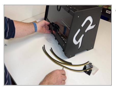
Install the latch plate for the seal kit as shown here. Optional Seal Kit Install Guide ID: 63 - Draft: 2021-12-25
