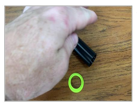
Press the roller flanges into each of the tubes as shown here.
