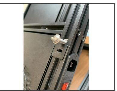
Temporarily add a screw to hold the slide nuts in place above the electronics tray brackets as shown.
