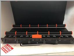
• If you have version 2.3 the "Parts Pack R" the "RollerSet wiht the Roller Flange from Parts Pack F will replace these steps. Just insert the flange inbetween printed tubes.
