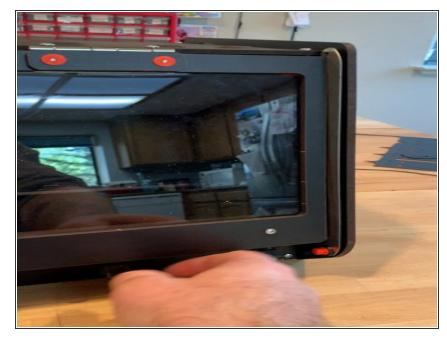
Another angle of the lid prop operation. Note the notch in the acrylic lid to hold the tip of the lid prop in place while the lid is open.
