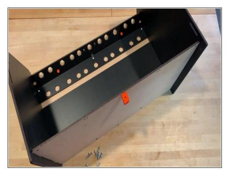
For the top rear corners you will only be using one fastener on the side of the bracket furthest away from the sidepanel to secure it to the back panel as shown.
