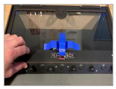
Start by removing the three screws with the thick washers installed during main assembly as shown here.
