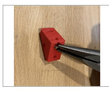
Bracket Preparation is absolutely critical to a frustration free and successful build. The time you invest now in making sure everything fits well and threads properly will make assembly go so much smoother and prevent possible damage to your brackets or RepBox.
