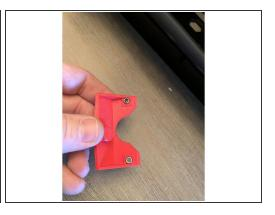
Press nylocks into nut traps of the latch plate as shown in pic 1
